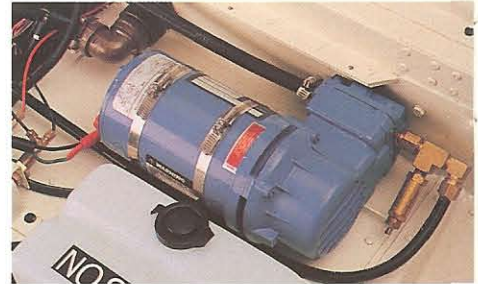
As part of the Central Tire Inflation System, the on-board compressor allows you to inflate or deflate your tires on the move for added traction and a smoother ride in harsh terrain.
