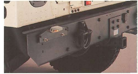
Optional Trailer Towing System allows your HUMMER to tow almost 9,000 lbs.
