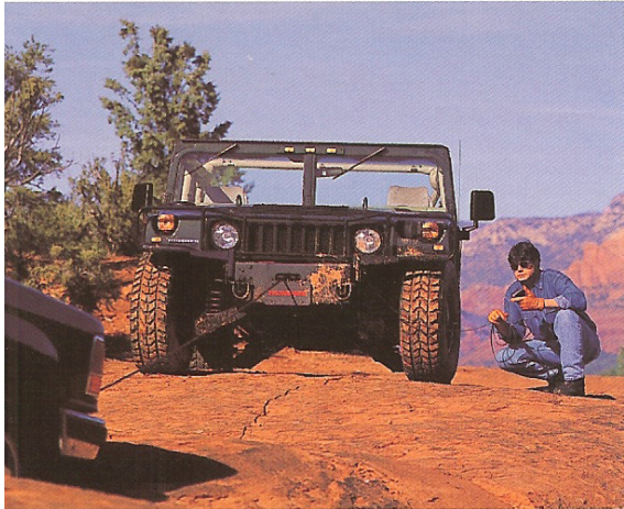
Optional electrically-powered, remote-controlled winch with 12,000-lb. capacity.
