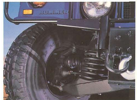
Geared hubs mean better mobility, and heavy-duty springs add to a more comfortable ride.
